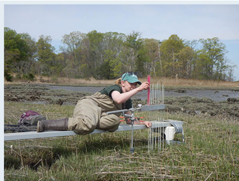
Habitat Coordinator Victoria O'Neill measuring the elevation change of coastal marsh sediment with a Surface Elevation Table at West Pond in Glen Cove, NY. Credit: NYSDEC.
